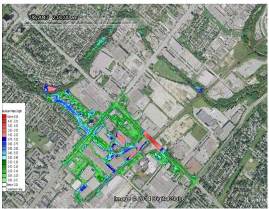
Maximum flood depth for 100year flood event with flood wall and berm implemented. © DHI
