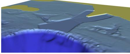
Model representation of the bathymetry of the seafloor at Falmouth cruise terminal, showing the steep drop at the reef edge as well as the dredged access channel.
