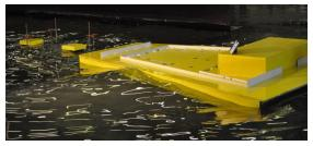
Testing a protective layout consisting of wave screens at our physical test facility.
