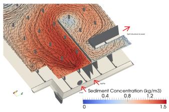
Close up of contour plot near the free surface for the model with a baffle included. The model has been spilling for 500 seconds. Surface vectors and streamlines show the location of the attachment of the inflow jet as well as the flow path around the baffle to the spill outlets. © DHI
