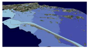
Range of flooded area (1,000 year return period discharge). Digital Terrain Model and Orthophotomap © Eurosense s.r.o. / Geodis Slovakia s.r.o. 2008-2011.
