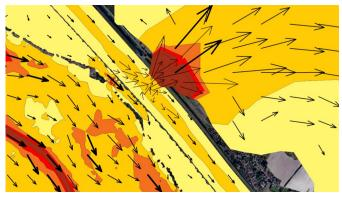
Detail of the current speed map with vectors showing flow direction (1,000 year return period discharge). Digital Terrain Model and Orthophotomap © Eurosense s.r.o. / Geodis Slovakia s.r.o. 2008-2011.
