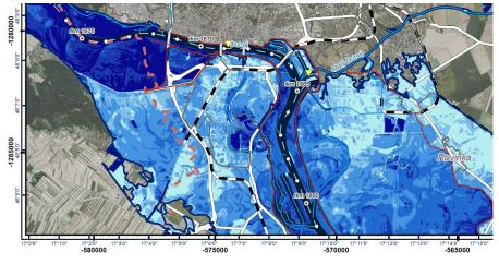
Flood hazard map list illustration of water depth (1,000 year return period discharge). Digital Terrain Model and Orthophotomap © Eurosense s.r.o. / Geodis Slovakia s.r.o. 2008-2011.
