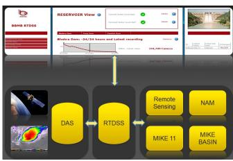
Schematic diagram showing data flow from sensors to database, models and decision makers.
