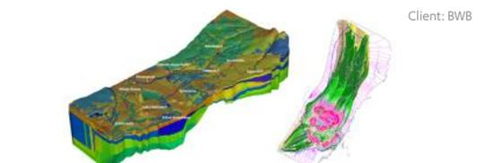
Underground oil and gas storage: Simulation of the dewatering process during the construction of storage caverns for liquefied natural gas (LNG), including seawater intrusion (density-dependent flow) and variably saturated flow. The work carried out dealt with complex geometrical and physical conditions. Within the project innovative solutions for the posed problems have been applied, including script developments that can also be applied in other subsurface construction projects.
