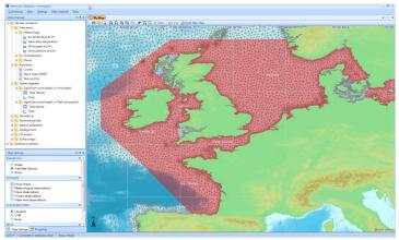
Database user interface with quick access and export functionality of MetOcean time series and analyses. This image shows a coarse representation of the computational mesh with more than 200,000 elements resolving nearshore areas with 1-3 km elements. ©DHI
