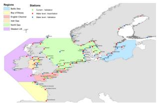
Geographical coverage of the database as well as locations of water level and current measurements. ©DHI
