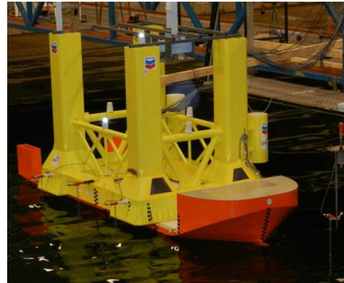
Testing the steel gravity structure transport in head sea.
