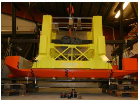
Joint heavy lift vessel and steel gravity structure model undergoing swing tests for transverse load characteristics.
