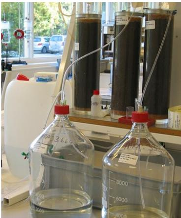
Column leaching tests performed on soil samples.
